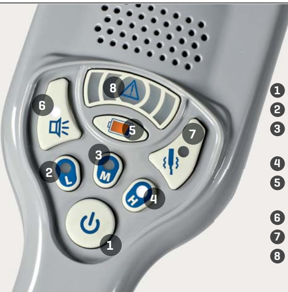
Optical indication proportional to the radioactive substance signal strength.
